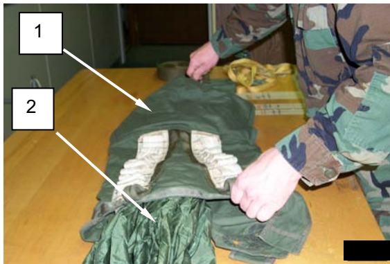
Figure 42. Stowing the Canopy.
