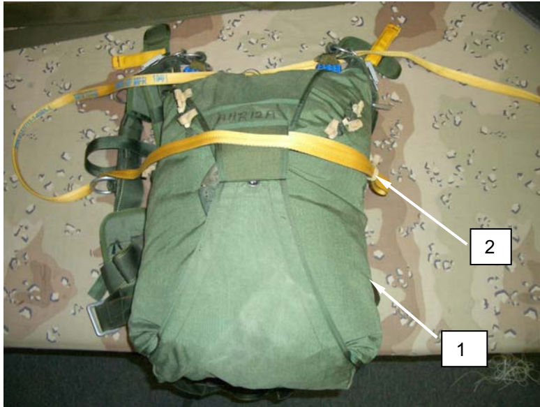
Figure 1. Lay Pack Tray On Pack Table.
