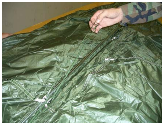
Figure 26. Dressing the Extended Gores. 0015 00-21
