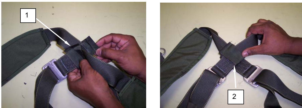
Figure 7. Replacing Harness Left Upper Main Lift Web (continued).
