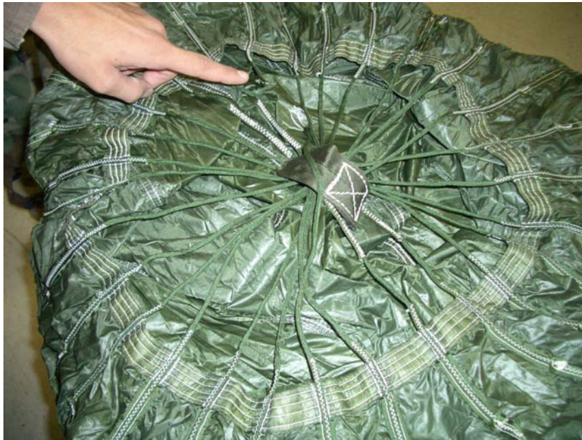
Figure 1. Main Canopy Vent Line Repair.
