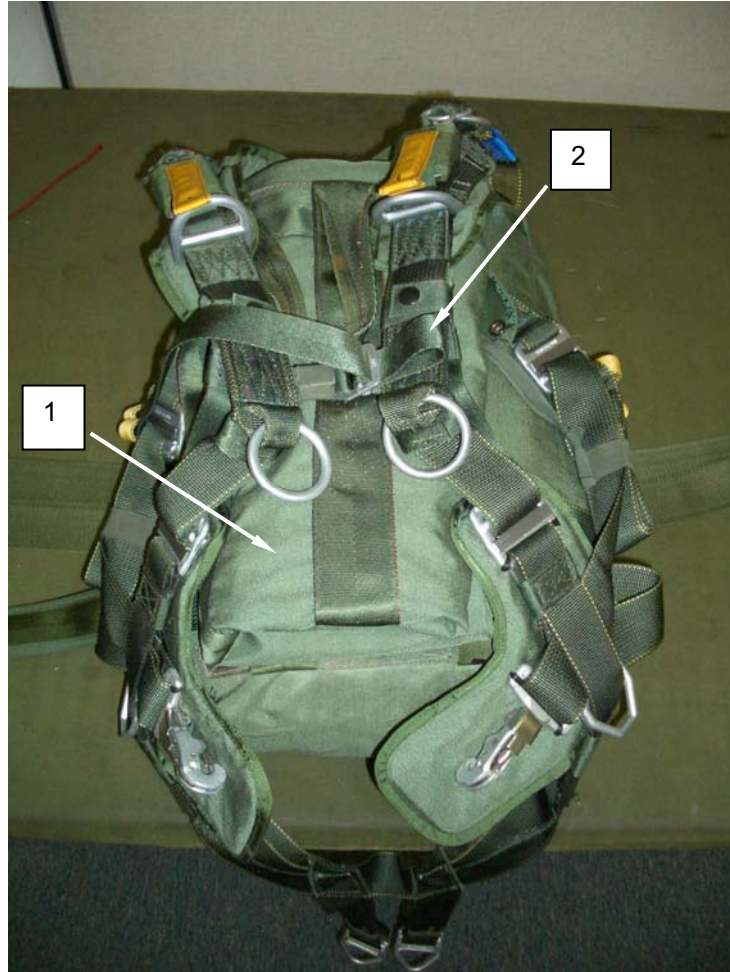
Figure 66. Folding the Harness.
