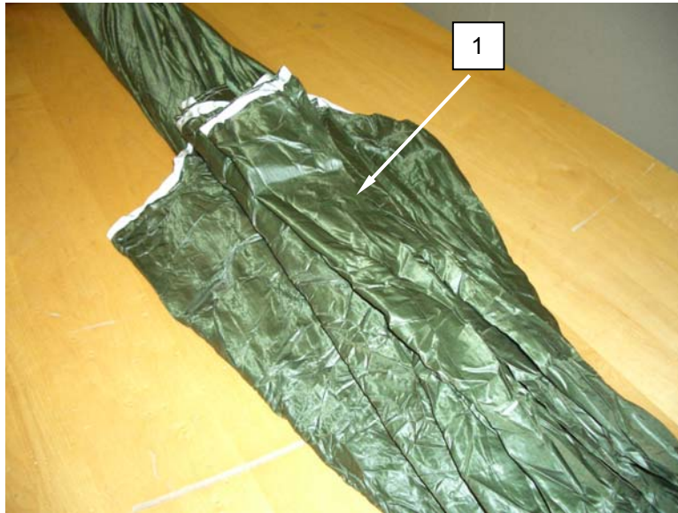
Figure 18. S-Folding Left and Right Side on top of the Folded Top Scoop.
