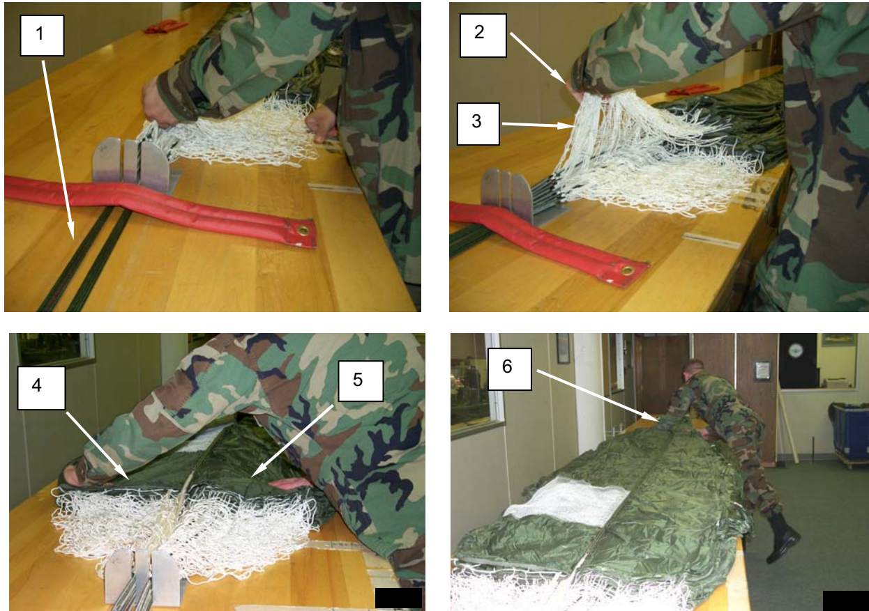
Figure 24. Separating the Canopy.
