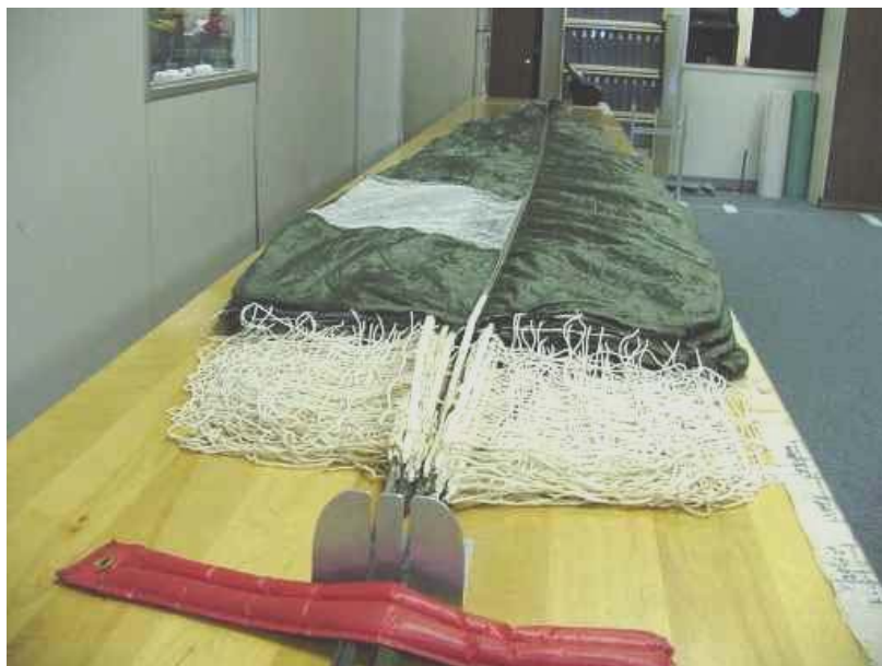
Figure 28. Canopy in Flat-Fold.
