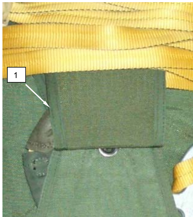
Figure 1. Replace Damaged Pin Protector Flap.
