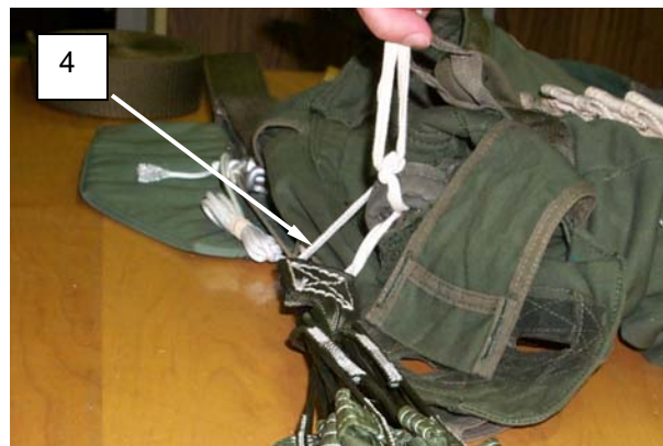
Figure 40. Securing Main Canopy Bridle Loop To Girth Hitch of Static Line.
