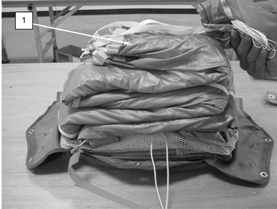
Figure 36. S-folding Remaining Canopy.
