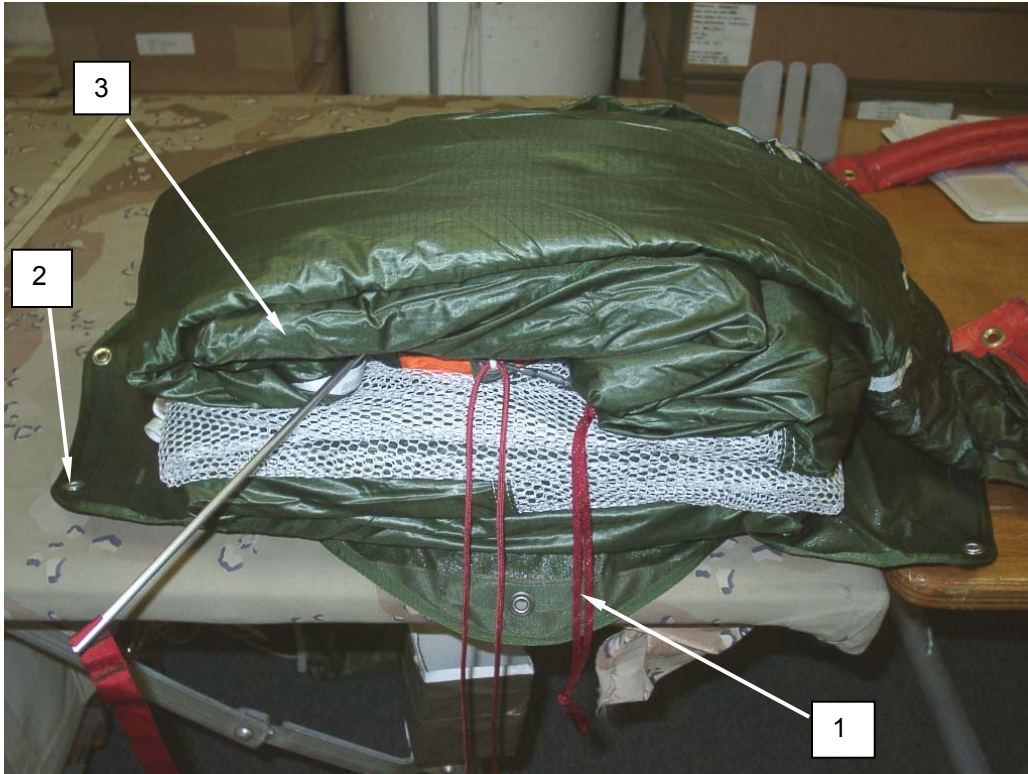
Figure 35. Forming a Bridge Over Top of Ejector Spring.
