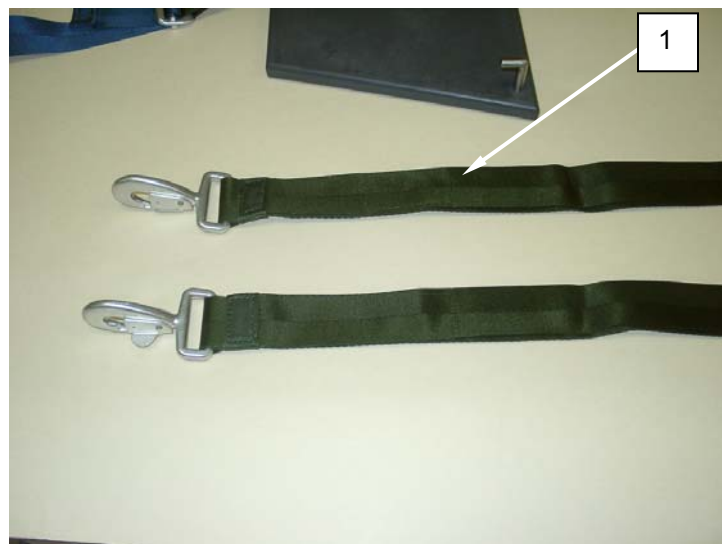
Figure 5. Laying Out Risers.
