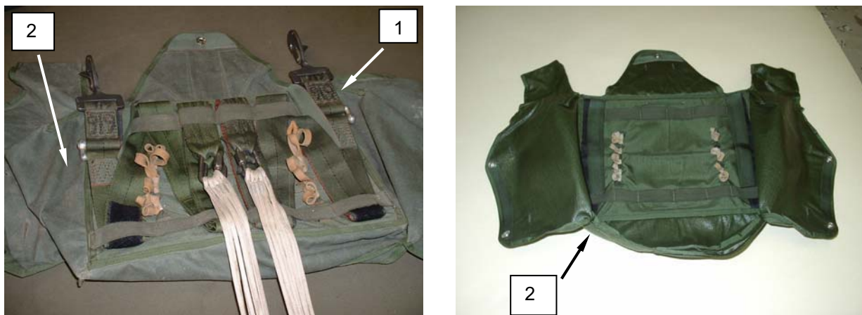
Figure 1. Remove Reserve Pack Tray from Reserve Canopy Risers.
