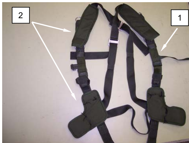
Figure 1. Replacing Harness Left Upper Main Lift Web.
