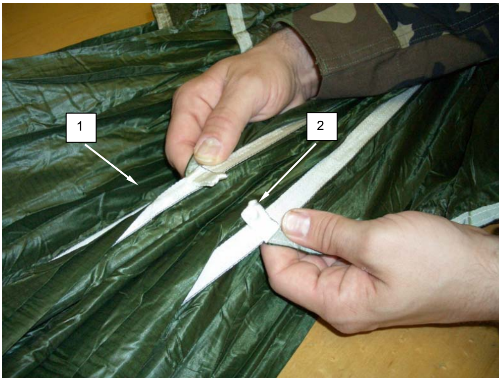
Figure 11. Tying the Apex Scoops.
