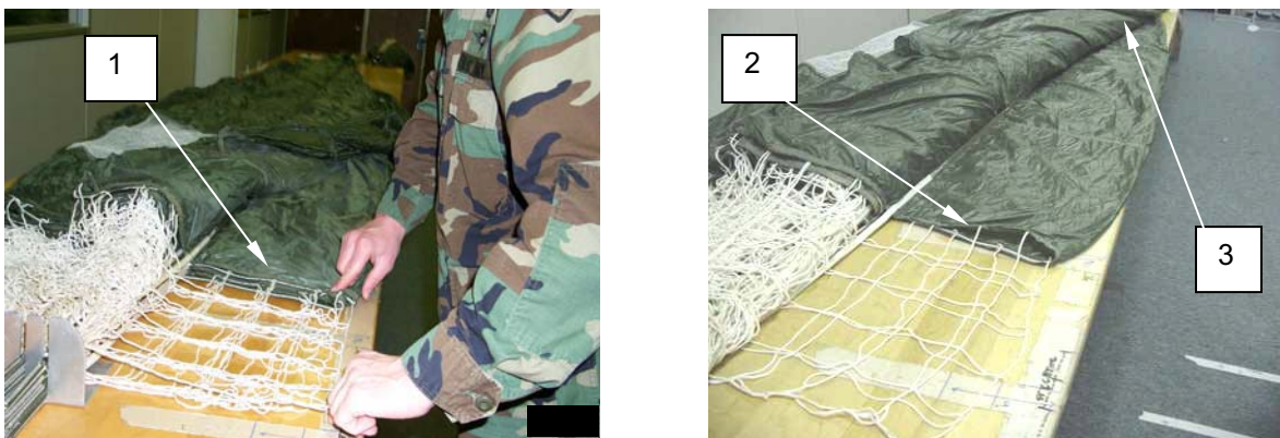
Figure 25. Fine Dressing the Bottom Gores.
