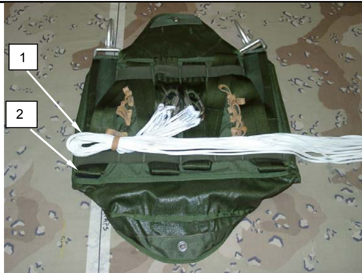
Figure 21. Making First Regular Stow.
