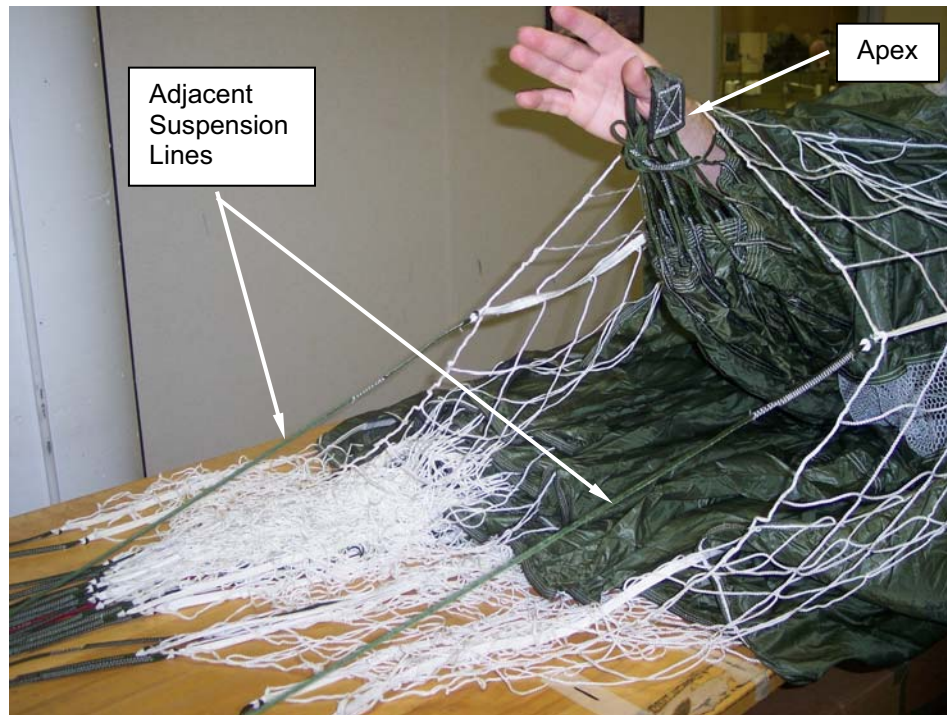
Figure 4. Removing An Inversion Through Skirt.
