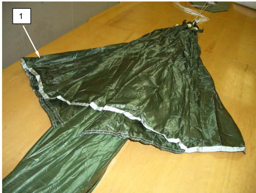
Figure 16. Dressing Left and Right Scoops.
